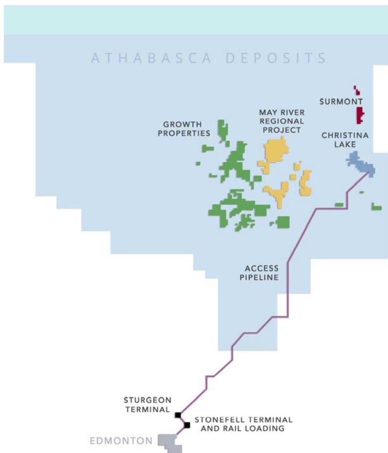
MEG's owned capacity in the Access Pipeline is currently approximately 200,000 bbls/d of blended bitumen and 87,000 bbls/d of condensate. MEG uses condensate as diluent. The blend line can be expanded through the addition of pump capacity as throughput requirements expand. The owners of Access Pipeline converted the system's former 24" blend line to diluent service in the third quarter of 2015.
