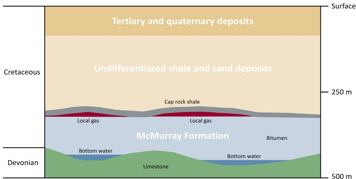
The unconsolidated sands of the McMurray at the Christina Lake Project are suitable for *in situ* recovery. The reservoir is situated at an average depth of 360 metres. The reservoir sand ranges in thickness from 9 - 56 metres with an average approximate thickness of 19 metres. Bitumen saturation is between 75% and 85%. Reservoir sands
